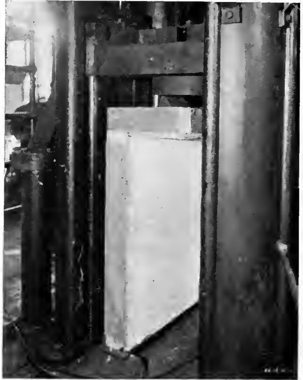
SHOWING TEST SAMPLE SUPPORTED ON END STUD
